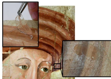
Fig. 15 The easy removal of the gel and its efficacy on the treated sample.
